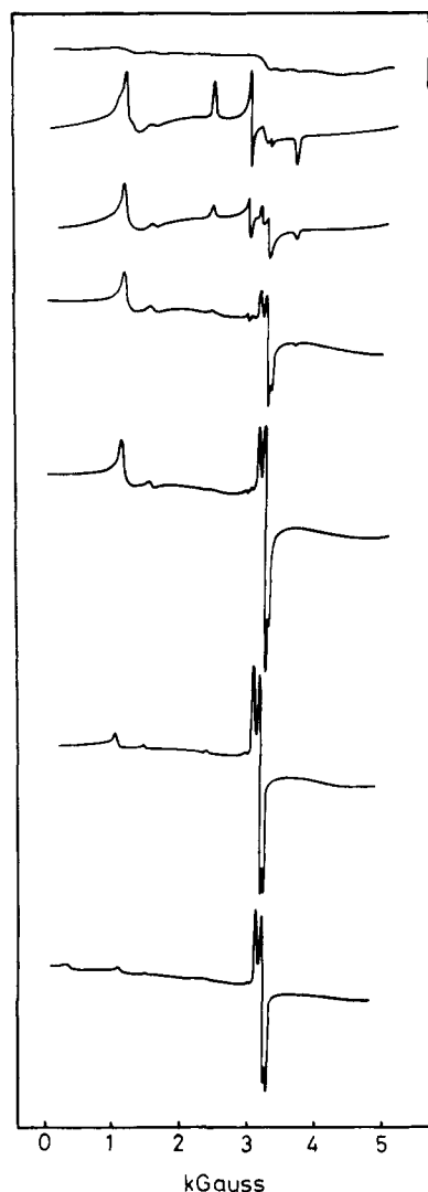
FIGURE 6: EPR spectra of mixtures of ccp and O -benzoylhydroxylamine, taken under the conditions described in the text. From the top, the samples contained: oxidant alone; ccp alone; 0.2 mol of oxidant/mol of ccp; 0.6 mol/mol; 1.1 mol/mol; 2.2 mol/mol; 4.4 mol/mol. The last two spectra were recorded with gain settings one-half and one-fourth that used for the first five spectra.
